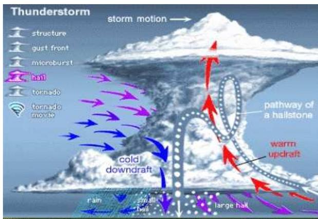
In order to prevent hail damages, it is necessary to transform the dangerous convective clouds so as not to allow the formation of large hailstones. Usually, the number of ice crystals in the cloud is small and, upon the existence of appropriate conditions, they grow rapidly to hailstones with large sizes.
