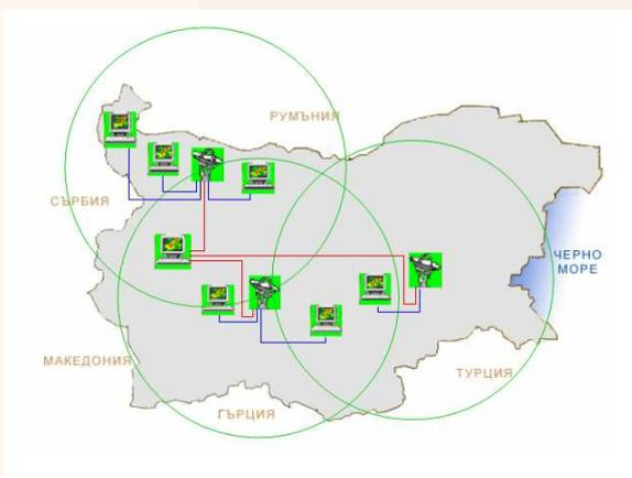
The Agency carries out its activities by monitoring the weather conditions using MRL5-IRIS Doppler radars and cloud seeding. Real time meteorological radar information is transferred to the National Civil Protection Service and the Air-Force.
